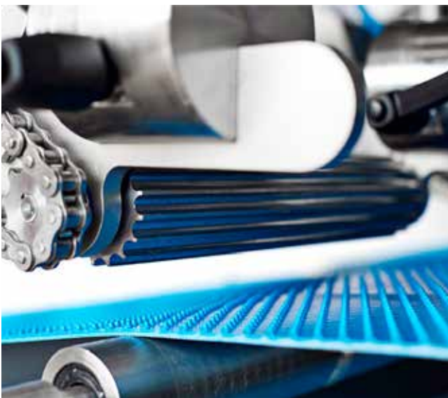
The raising rollers are perfect when processing very fresh fillets.
