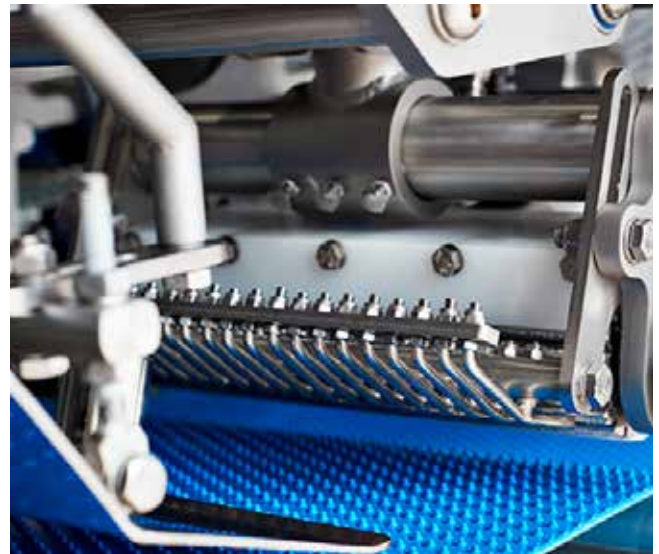
The in-feed roller guide system is the option you need when processing fillets with very slippery skin.
