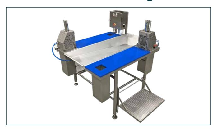
Manual deheading requires the best working conditions. The de-head table is designed for the efficient de-heading of fish while considering ergonomics.
