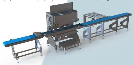
Each product is measured by a high quantity of lasers to determine its physical size and direction on the belt. A proportionate amount of salt is applied specific to each side's location (belly/loin side left or right).
