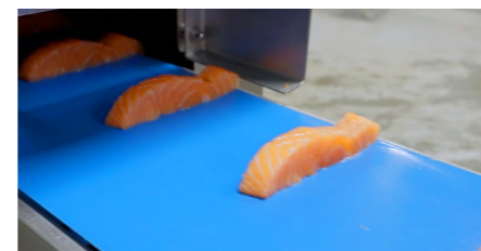
The fillet is first cut into precise slices and then enters a second stage where it is cut into cubes
