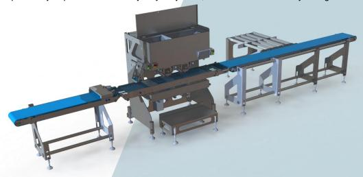
Each salmon is measured by a high quantity of lasers to determine its physical size and direction on the belt. A proportionate amount of salt is applied specific to each fillet's location (belly side left or right). The machine can also double as a spice doser and combine salt and spice as in production of gravadlax.
